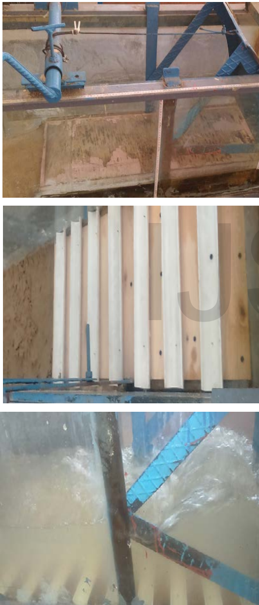
Fig. 1 the different materials used downstream the radial gate, and the jump over corrugated bed.
